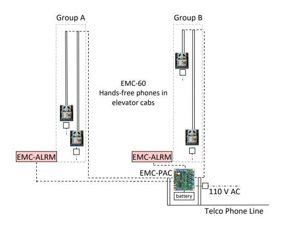
\_\_\_\_\_ Shielded Twisted Pair (STP)
